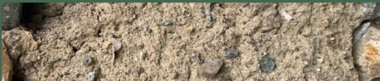
Eroded tempered clay exposing aggregate.
